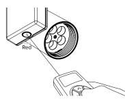
4 To complete the process, hold the 🕥 button and aim the laser away from the sensor. The LED on the spotlight will flash green to indicate that the Start Address has been received.
