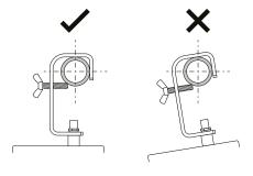
For multiple fixtures, ensure that hook clamp orientation is the same for each mounting.
