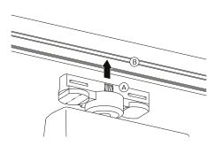
Rotate tab © clockwise 90° to connect the adaptor to the neutral circuit.
