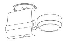
The monopoint fixture requires a *minimum* clearance distance of 200mm above and around the mounting point and a maximum ceiling material thickness of between 3mm and 35mm.
