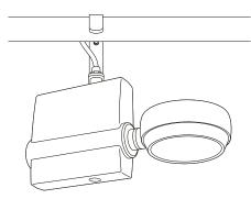
The hook clamp fixture fits barrel bar with a minimum diameter of Ø40mm and a maximum diameter of Ø50mm.
