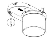
4 Insert the bezel ring over the snoot and clip into place over the accessory ring to lock the assembly together. Reattach the assembly to the DR8 spotlight.
