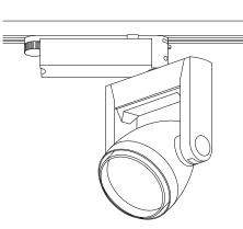
Ensure that the track system where the DR8 luminaire is to be installed is compatible with the Eutrac 1-Circuit adaptor.
