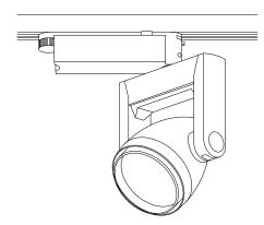
Ensure that the track system where the DR8 luminaire is to be installed is compatible with the Eutrac 2-Circuit adaptor.
