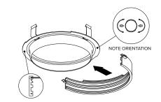
3 Insert the snoot into bottom slot of the accessory ring, as shown and bring the two halves of the ring together.
