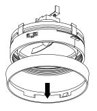
3 The accessory holder can hold up to two lenses, depending on the lamp type.
