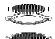
Insert the accessory holder up through the DRX5 face plate and magentically attach to the optic holder.
