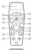
**OLED Display** 2 Global Command Pan Left Select (Activate Laser) Dim Up Dim Down Lamp On/Off Tilt Up Pan Right Tilt Down Function Up Confirm/Send Function Down Back Laser Infrared Diode
