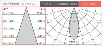
BEAM DIAMETER AT 10M: 6.1M
