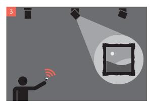
**3.** When the adjustments are complete, press the laser button to deselect the luminaire.
