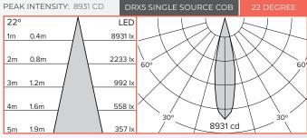
BEAM DIAMETER AT 10M: 1.8M
