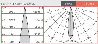
LX AT 10M: 320 LX BEAM DIAMETER AT 10M: 3M
