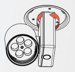
Twist the luminaire clockwise until it stops.
