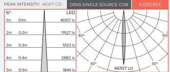
BEAM DIAMETER AT 10M: 0.7M
