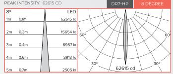
BEAM DIAMETER AT 10M: 1M
