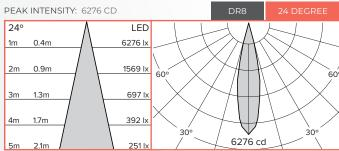
BEAM DIAMETER AT 10M: 4.3M
