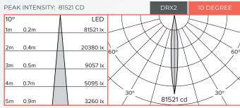
BEAM DIAMETER AT 10M: 1.8M
