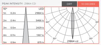
BEAM DIAMETER AT 10M: 1.8M
