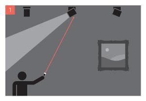
**1.** Select the RCL luminaire you wish to control with the RCL handheld remote's built in laser\*.
