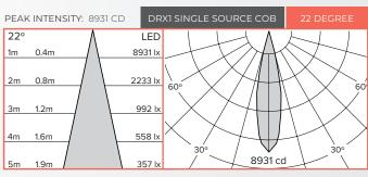
BEAM DIAMETER AT 10M: 3M
