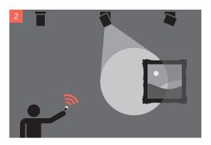
**2.** Once the luminaire has been selected, colour temperature, beam width, dim level and beam positioning can be altered using the remote.
