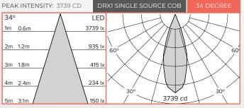
BEAM DIAMETER AT 10M: 6.1M
