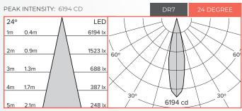
BEAM DIAMETER AT 10M: 6.1M
