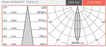
BEAM DIAMETER AT 10M: 3M
