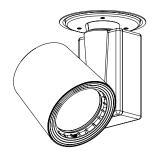
The monopoint fixture requires a minimum clearance distance of 200mm above and around the mounting point and a ceiling material thickness of 3-35mm.
