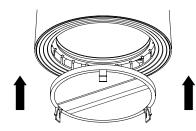
To fix the accessory clip safely in place, push it through the optic face until all 3 clips snap into place.
