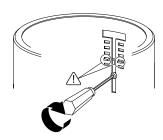
8 Ensure that the luminaire is securely installed, with the fixing clips firmly against the ceiling material.
