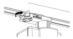
Rotate tab (D) to the desired circuit position
