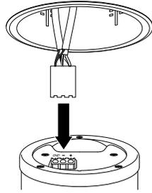
12 Insert the control gear through the mounting ring onto the upper surface of the ceiling.
