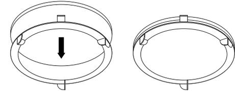
2 Using the finger grips on the outside of the clip, raise the accessory into the can of the DRX1 until it meets the LED module.
