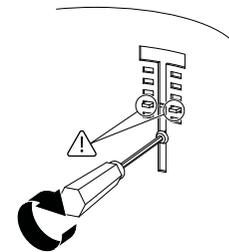
8 Ensure that the luminaire is securely installed, with the fixing clips firmly against the ceiling material.
