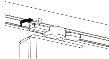
5 With the 3-Circuit track adaptor, you can choose which circuit the luminaire is connected to:
