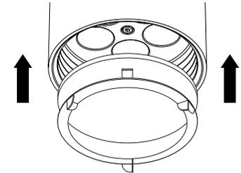
3 To hold the accessory clip safely in place, rotate it clockwise until it locks with the fitting.
