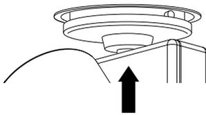
14 Twist spotlight clockwise and pull down gently to lock in place.
