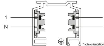
2 To mount the track adaptor into the track system, check that both tabs on the adaptor are in the open position and insert into the track.
