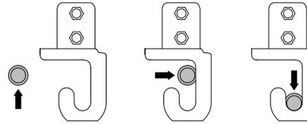
16 For multiple fixtures, Align primary hooks (denoted by a directional arrow) perpendicular to a feature such as a wall or trough edge to ensure all fixtures will align.
