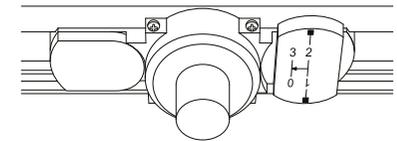
Circuit 1 - From the starting position, rotate the tab clockwise 90°.
