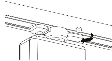
4 Rotate tab (D) to the desired circuit position (see section 5).
