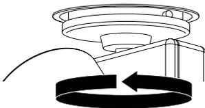
15 Ensure that the monopoint head studs locate securely in the mounting ring hooks, as shown below.
